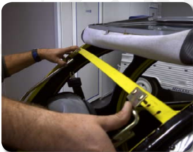
7/ Put down the upper bar with the hinges, screw the hinges with the washers and the nuts M5 ( number 8 spanner ).
