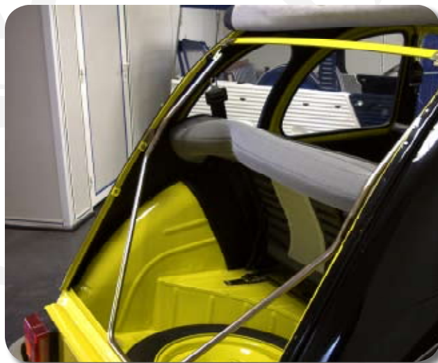
6/ Put on the upper bar ( ref 2202200 ) the left hinge ( ref 2202204 ) and right ( ref 2202206 ).
