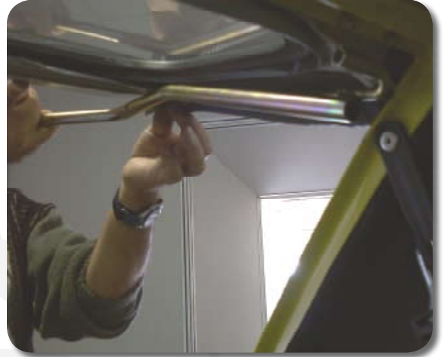
12/ Fix with the 5x25 screws the upper bar on to the roof crossbar inside the holes.
