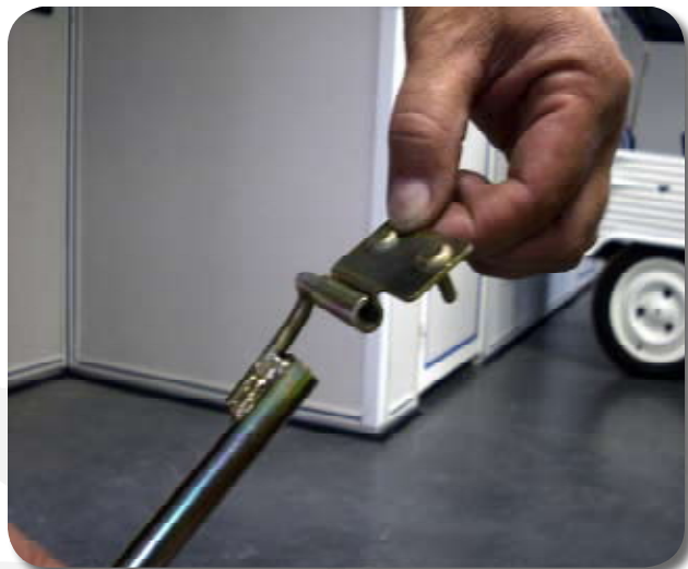
6/ Put on the upper bar ( ref 2202200 ) the left hinge ( ref 2202204 ) and right ( ref 2202206 ).
