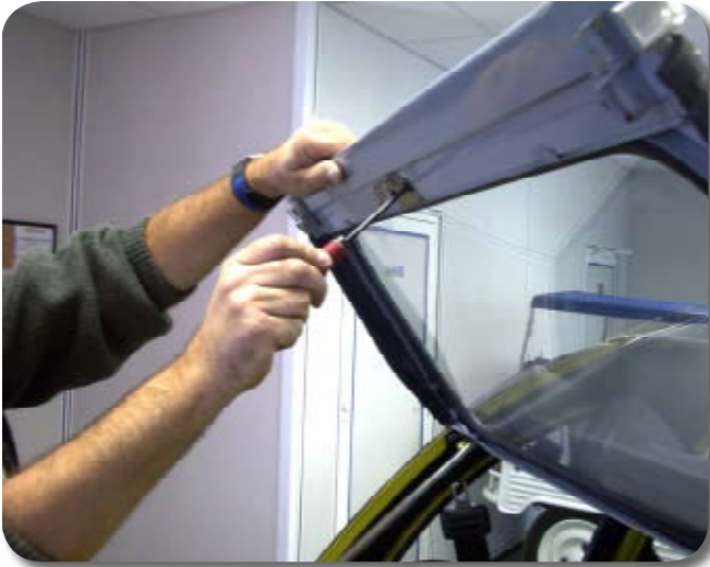
11/ Fix the open part towards the front of the vehicle to the centre of the roof crossbar with 2 metal screws.
