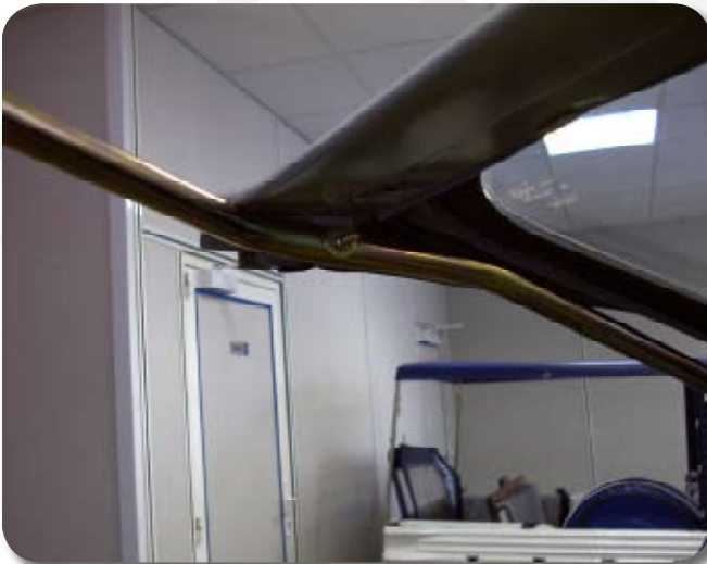
11/ Fix the open part towards the front of the vehicle to the centre of the roof crossbar with 2 metal screws.
